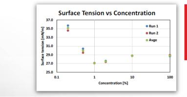
A 1% EndoTherm solution is the critical micelle Concentration with a mean surface tension of 27.1 mN/m
