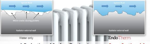
A Reduction of Surface Tension Increases Cross-Sectional Area Alters heat transfer coefficient EndoTherm Increases the Overall Heat Transfer Coefficient
