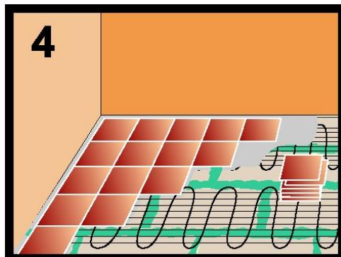
Place the heating mat accordingly for the desired heating area. Apply a layer of flexible sealing cement onto the heating mat and then place the floor tiles. Follow the instructions for their use when laying the heating mats (cables). The expansions joints in the surface finish must not be immediately above the corresponding spaces between the F-boards. The underlying expansion joints must be preserved.
