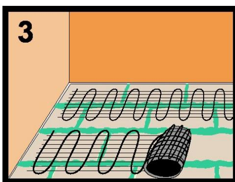
The spaces should be covered with a reinforcing gauze fabric tape. Place the tape, apply hydroinsulation adhesive material, spread the residual material with a spreader or remove it. The tape should overlap at least 50 mm. The boards don't have to be protected with additional hydroinsulation. Allow the adhesive material to harden, as described in the instructions for use.
