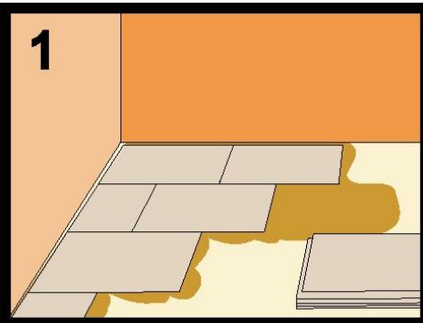
Spread the adhesive sealing cement with a notched spreader on the cement base. Place the boards as shown in Picture 1, setting and aligning them properly. Allow the adhesive material to harden, as described in the instructions for use. When laying the boards, the adhesive material must not come into the spaces between the boards. The expansion joints in the foundation must be preserved.
