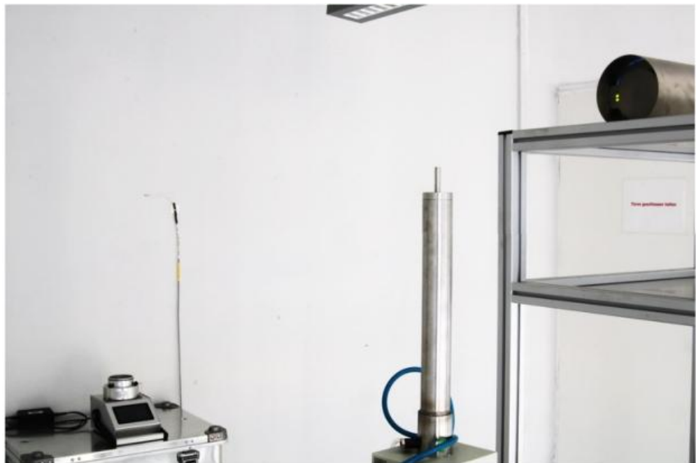
Figure 1: The (test) setup consisting of the air purifier (Freshair), a dosing unit and an air sampler in the testing room.
