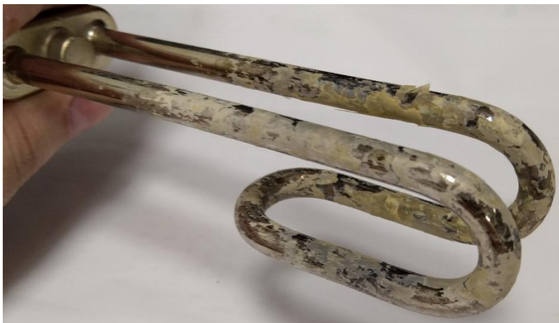
Pic. 2 The heating element from container 1 without water treatment.
