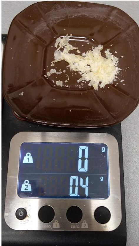
Pic.. 3 Measured weight of deposits from the electrode (left) and from the sediment at the bottom of the container (right).
